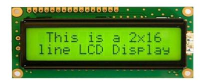
Fig.6.16\*2 LCD Display
