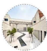
Water bodies in courtyard: Evaporative cooling as well as minimizing heat gain
