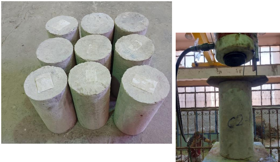
Figure 6. Cylinders Specimens and Test Setup
