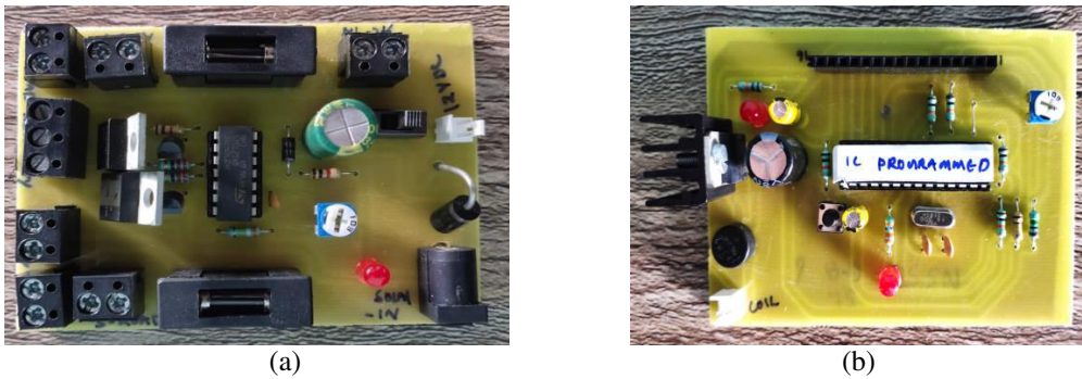
Fig.3. Printed Circuit Board (a) Solar Charger Controller (b) Microcontroller PCB
