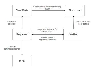
Fig. 2. System architecture
