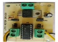
Fig.d Motor Driver Module – L293
