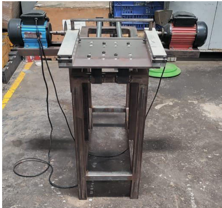
Figure 7: Ad Blue (DEF) Plastic Pipe Cutting Machine
