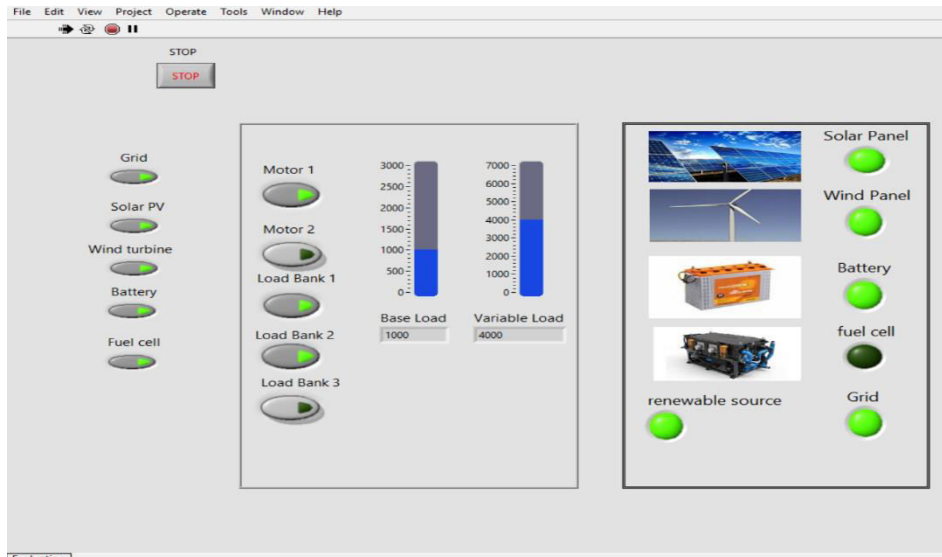
Fig. 7. One Motor and Two Load Bank are Turned ON
