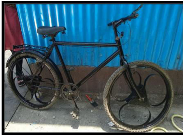
Fig 5.1 Loop Wheel Bicycle Construction
