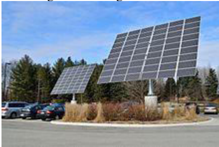
Solar modules mounted on solar trackers
