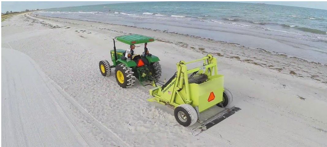
Fig.1.4: Surf Rake : Tractor towed beach cleaner machine.
