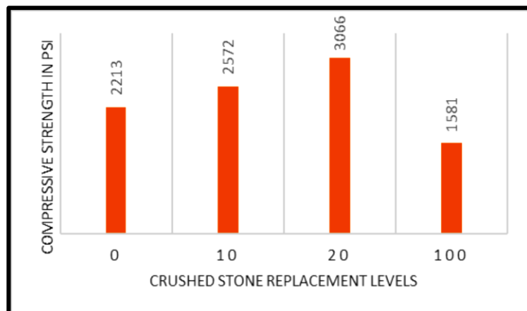
Fig 2: Compressive strength values at 7 days curing period.
