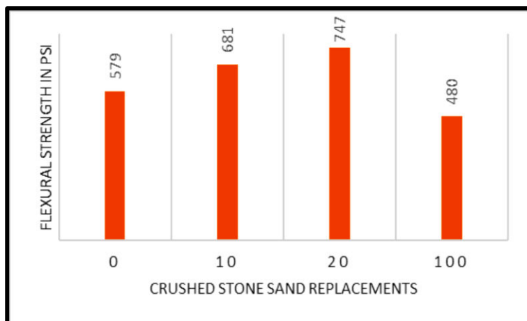
Fig 7: Flexural strength values at 28 days curing period.
