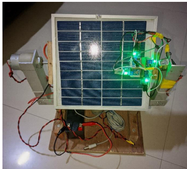
Fig7. Solar Tracking System
