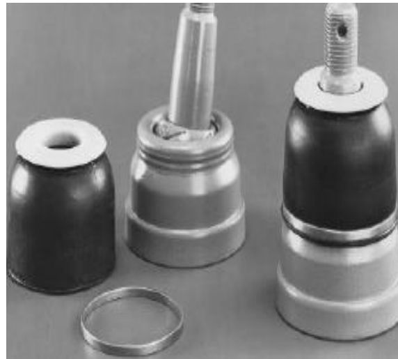
Fig.1 The first industrial component manufactured using the electromagnetic forming process.
