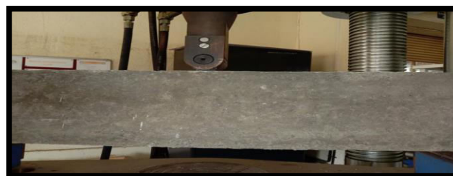
Fig. 3 One point loading
