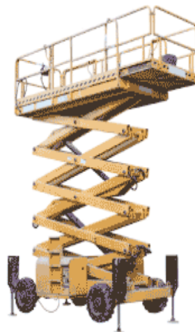
Figure 2: Prototype of Hydraulic lift
