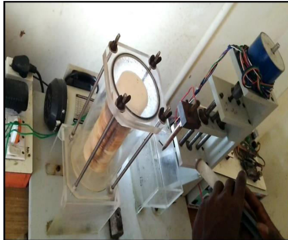
Figure 3.1 ECMM Setup Working principle of ECMM
