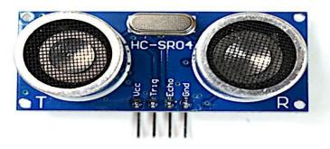
Fig 4: Ultrasonic Sensor
