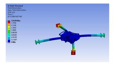
Fig 4.4 Deformation of 1.95mm
