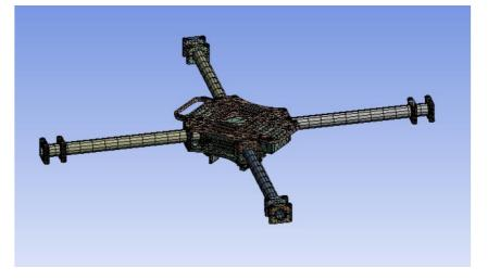
Fig 4.2 Mesh Model Drone Ansys
