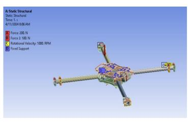
Fig 4.3 Load and Boundary condition applied to Object
