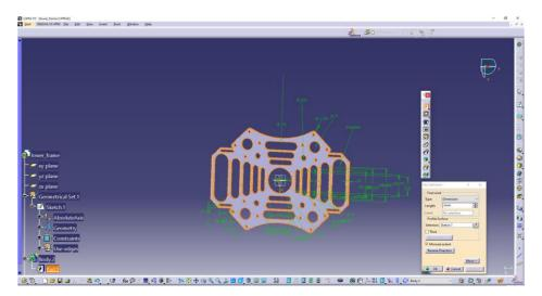
Fig 3.4.2 Part Design for Lower Frame
