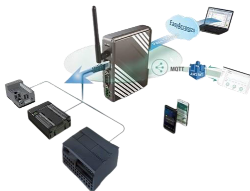
Fig. 2. PLC integration with Weintek HMI
