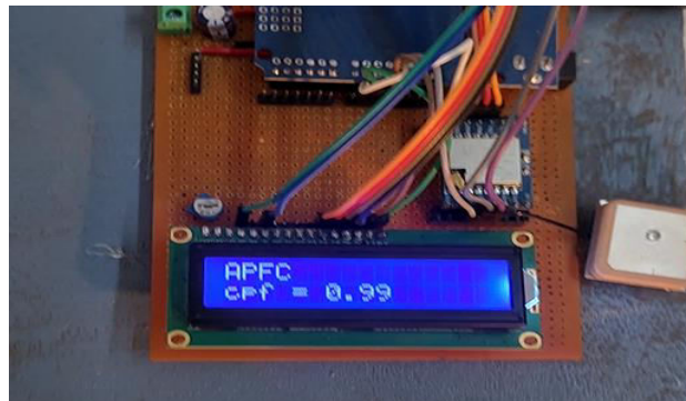
FIGURE 7. POWER FACTOR AFTER RESISTIVE LOAD ON
