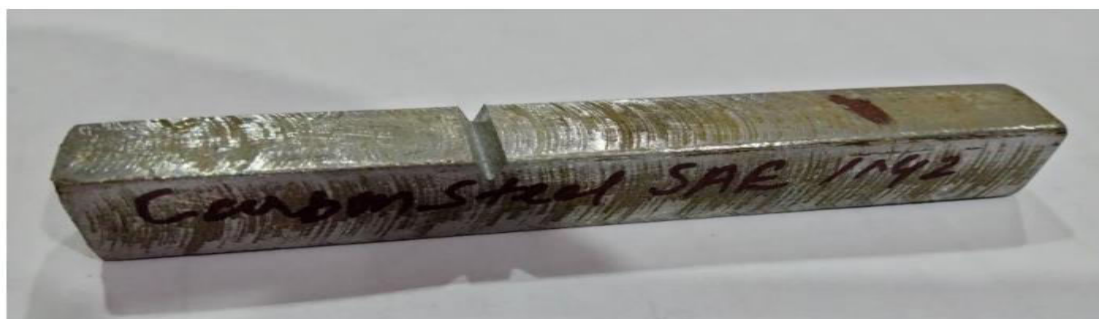
Fig. 2: Izod Specimen of Carbon Steel SAE 1042
