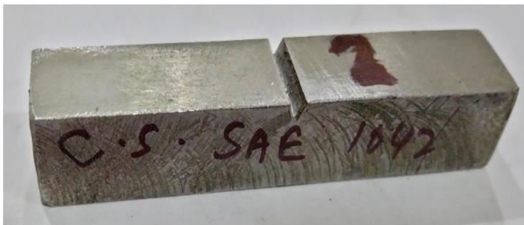
Fig 6: Charpy Test Specimen of Carbon Steel SAE 1042
