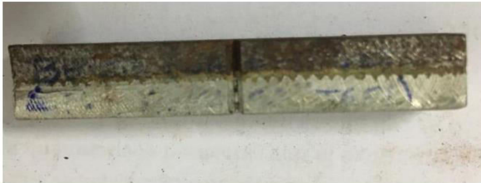
Fig 8: Charpy Test Specimen of CS + Epoxy + Aluminium 5083 H112
