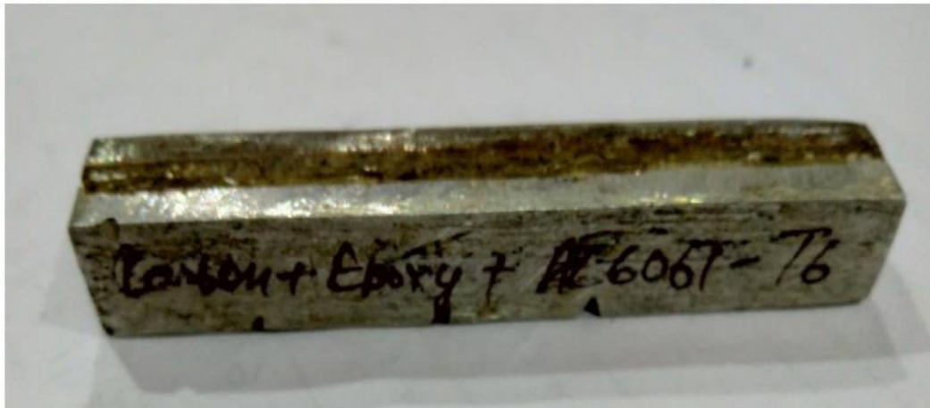
Fig 4: Izod Specimen of Carbon Steel SAE 1042 + Epoxy + Aluminium 6061 T6
