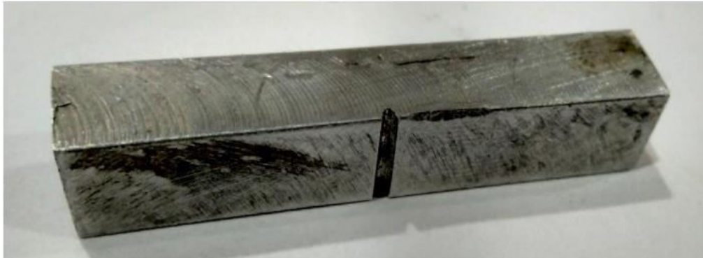
Fig 7: Charpy Test Specimen of Aluminium 6061 T6
