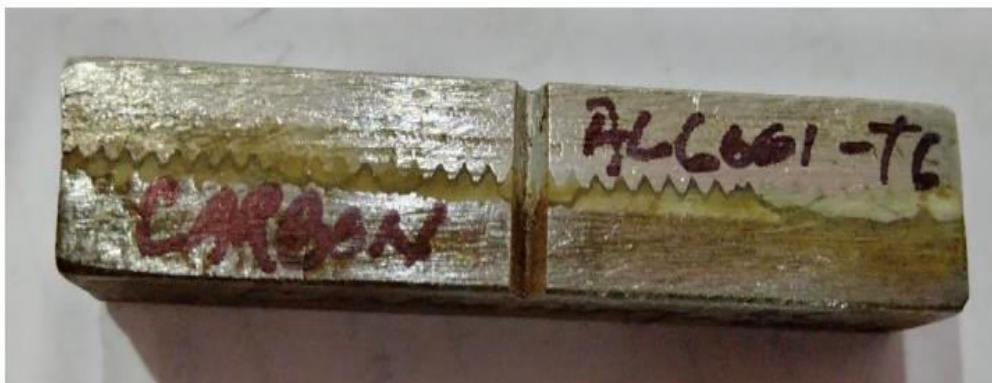
Fig 9: Charpy Test Specimen of Carbon Steel SAE 1042 + Epoxy + Aluminium 6061 T6
