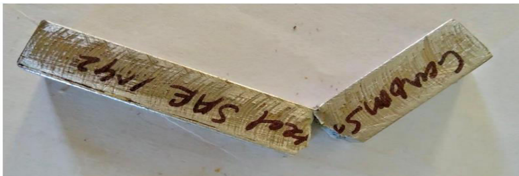
Fig 5: Carbon Steel SAE 1042 Specimen after test was performed
