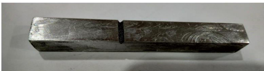
Fig 3: Izod Specimen of Aluminium 6061 T6
