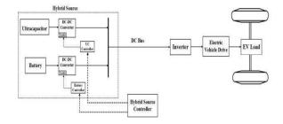
Fig.1hybrid source's overall interface block diagram with the EV load
