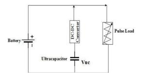
Fig. 3. Passive HESS system using a parallel combination of batteries and ultra capacitors
