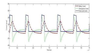
Fig. 4. Current distribution of the pulse loads from batteries and ultra capacitors in passive HESS
