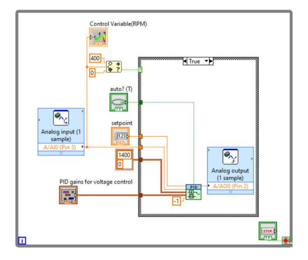
Fig 4 . Block Diagram of labview Program
