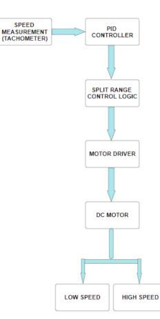
Fig 2. Block Diagram of Simulation Model
