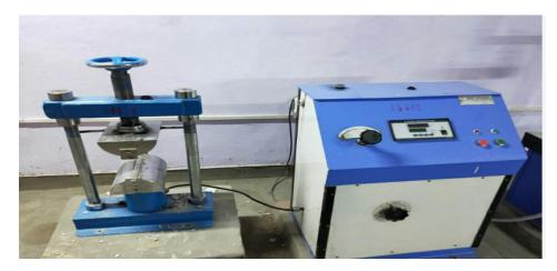
Fig.5 Split Tensile Strength Test Machine
