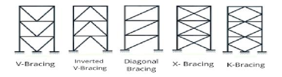
Fig.1 Different types of Bracings
