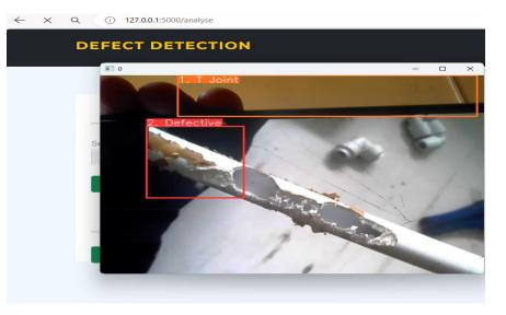
Fig(e): Result Showing the Defective Part using Live Image
