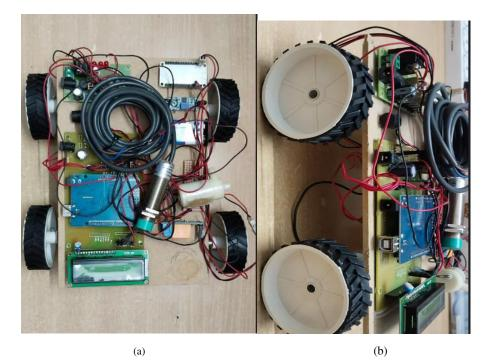
Fig. 2 Metal Fire Bot (a) Top View of the robot (b) Side View of the robot
