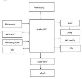
Fig. 1. System Architecture.
