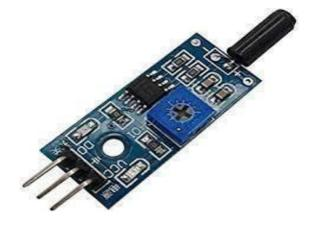
Figure 5 Vibration sensor
