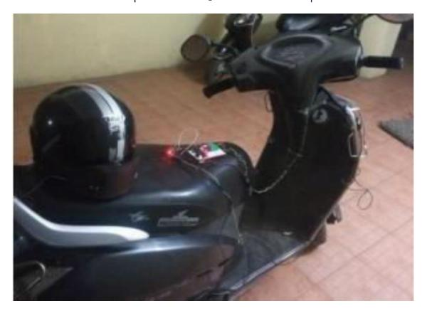
The best part about this project is that it doesn't work until it's worn since a limit switch has been added inside the helmet. Therefore it doesn't send messages if it thrown or falls down Also it's calibrated such that it won't send messages for values due to speed breaker's a other small knocks
