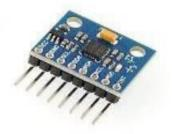
Figure 4 Gyroscope sensors
