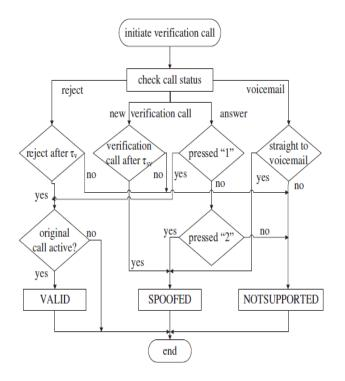
Figure 2. This flowchart shows how CallerDec handles different cases to detect caller ID spoofing. A new incoming call initiates the verification process.
