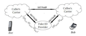
Figure 1. An illustration of how a fake ID provider spoofs a caller ID leveraging the loophole in network interconnection protocols.
