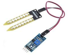
Fig 3 Soil moisture sensor
