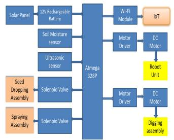
Fig1.Block Diagram of Proposed System
