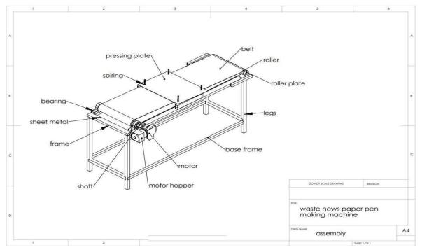
Fig 2.9 Assembly with labeled parts
