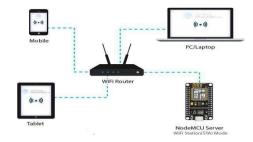
(e). ESP8266 as HTTP Server using Wi-Fi Access Point (AP) mode.
