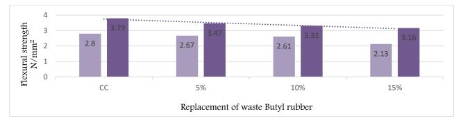
Figure 3. Graphical representation of Flexural strength at 7 and 28 days
