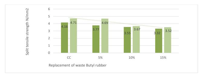
Figure 2. Graphical representation of Split tensile strength test at 7 and 28 Days
