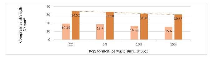
Figure 1. Graphical representation of Compressive strength test at 7 and 28 Days
