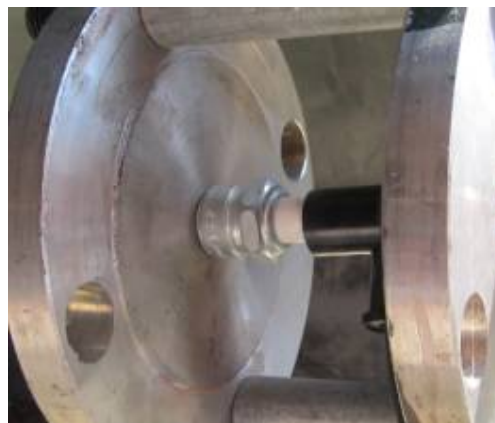
Fig. 4: Igniter plug mounting on flange
