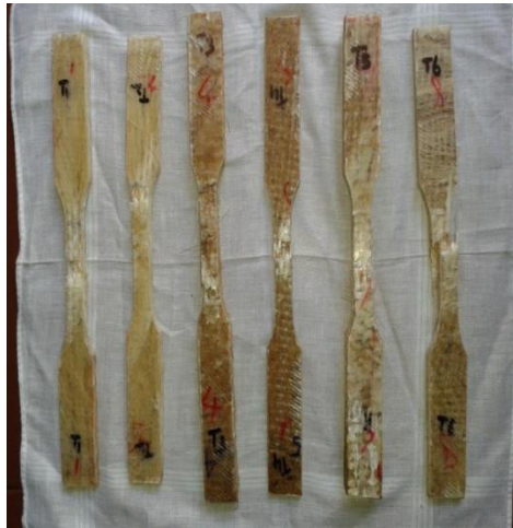
Fig 5: Tensile test specimen
