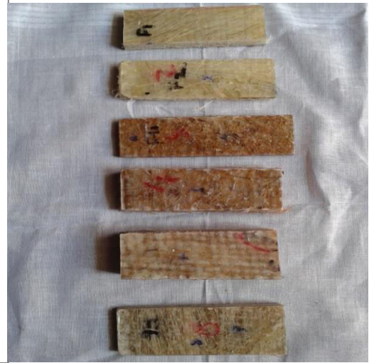
Fig 9: Flexural test specimen
