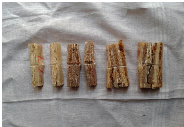
Fig 10: Impact test specimen
