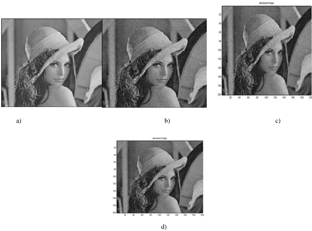
Fig. 4 a) Original b) Fig. 5 Noisy image ( \sigma = 20\text{dB} ) c) .Denoised image ( \sigma = 20\text{dB} ) , PSNR =28.99dB,MMSE Method d) Denoised image ( \sigma = 20\text{dB} ) ,PSNR =30.34dB, Modified stochastic Method(Our Method)
