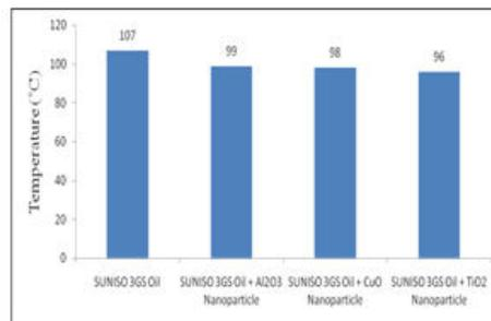
**FIG.6. TEMPERATURE OF THE COMPRESSOR DOME**
