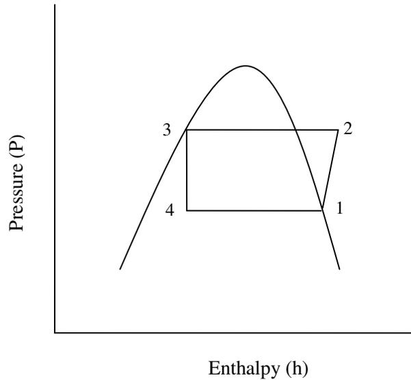
**FIG.5. P-h diagram of a V.C. Refrigeration System**
