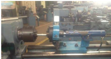
FIGURE 4. FRICTION WELDING SETUP
