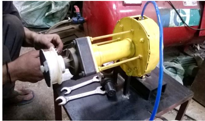
Photo 1:- Photo of Quasi turbine rotary air engine
