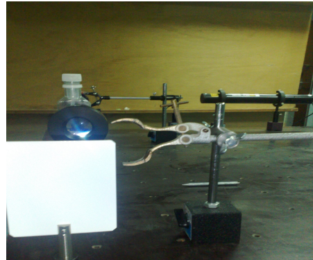
Fig. 1 Digital holography setup and apparatus for deformation analysis.
