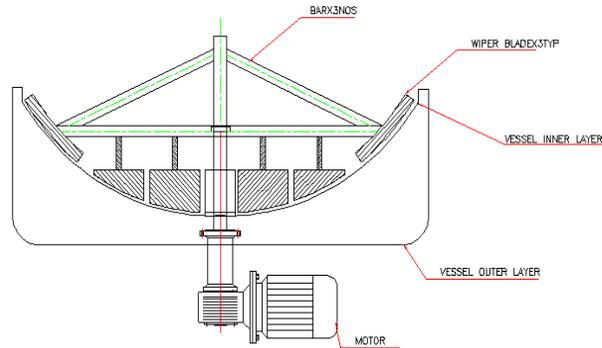
Fig 4 (c) Paddle Agitator Assembly
