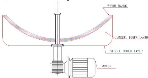
Fig.4 (b) Paddle Agitator Assembly
