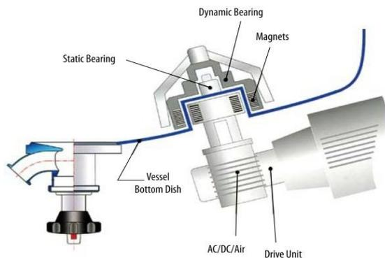
Figure.4.(e) Magnetic Motor
