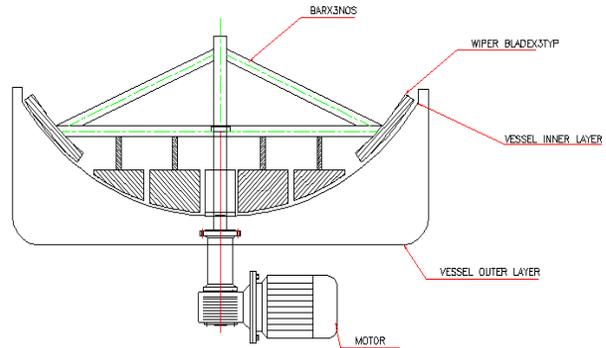
Fig 4 (c) Paddle Agitator Assembly
