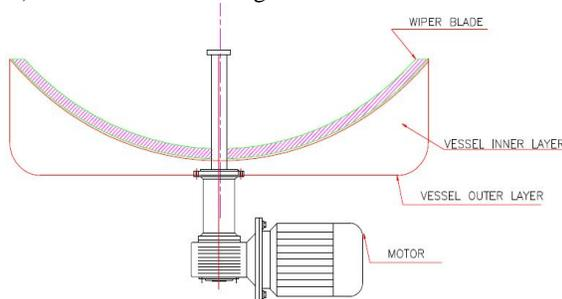
Fig.4 (b) Paddle Agitator Assembly
