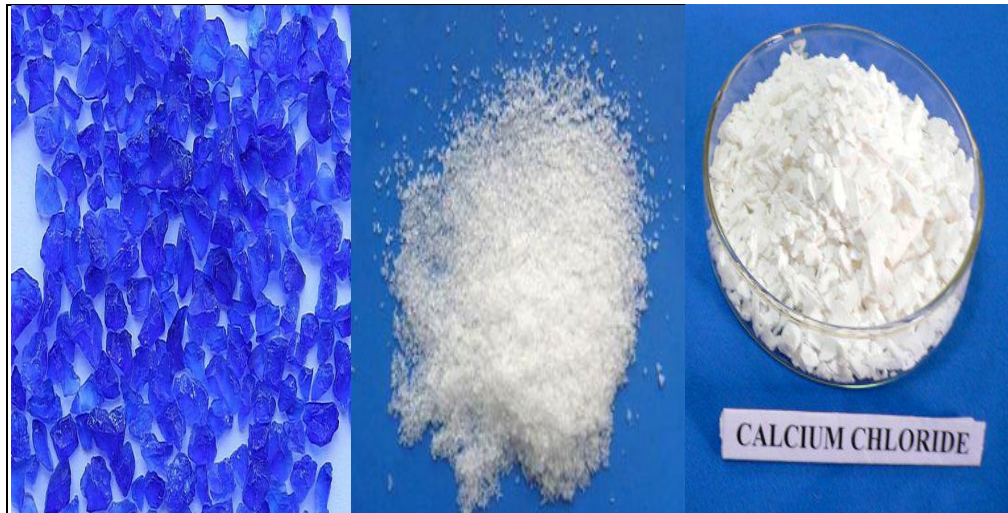
Fig. 1 Desiccant Materials Used (a) Silica Gel (b) Magnesium Sulphate (c) Calcium chloride
