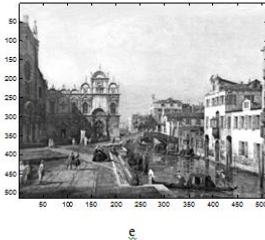
Fig. 1 Image denoising (a) Original image (b) noisy image( \sigma=30 ) (c) de-noised image using new thresholding function with Translation invariant method (d) de-noised image using new thresholding function with Top method (e) de-noised image using new thresholding function with Universal method
