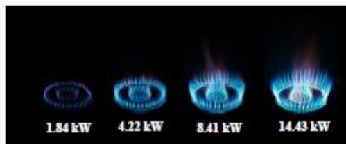
Fig 4. Effecting of heat input on flame structure for without preheats case [2]
