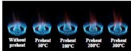
Fig 5. Effecting of primary air preheat on flame structure at q = 8.41 kW [2]
