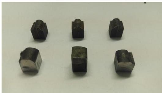
Fig. 3 Wear test specimens
