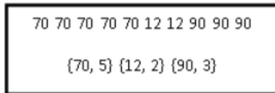
Fig3 Run length encoding
