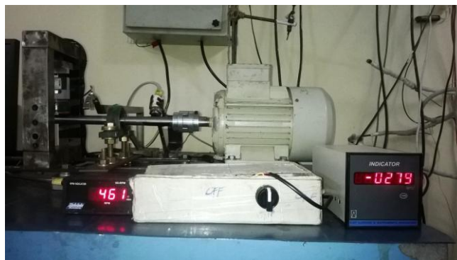
Fig. 7) Shaft is running at 461rpm and load capacity is 279 grams with impulse
