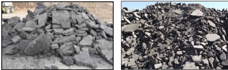
Fig: 2 Various Stockpiles of larger size RAP materials
