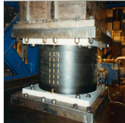
Fig 8. Force-displacement curve for Lead Rubber Bearing Fig 9. Actual photograph of installed Lead Rubber Bearing system.
