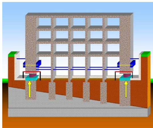
Fig 11.4 And thus the base isolators are installed.
